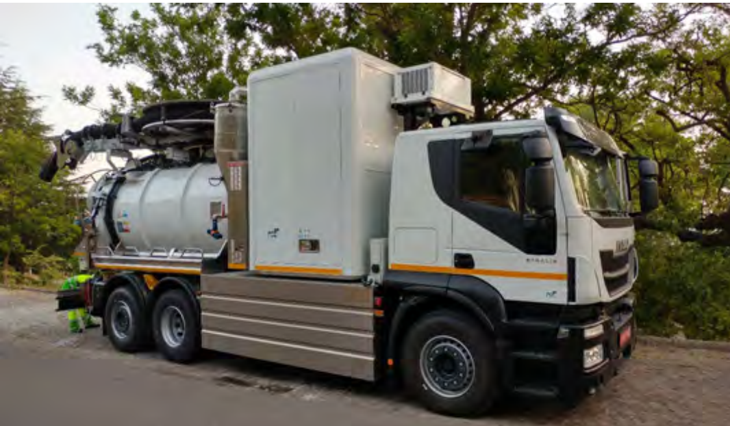
100% electric sewer system suction equipment in Barcelona.
